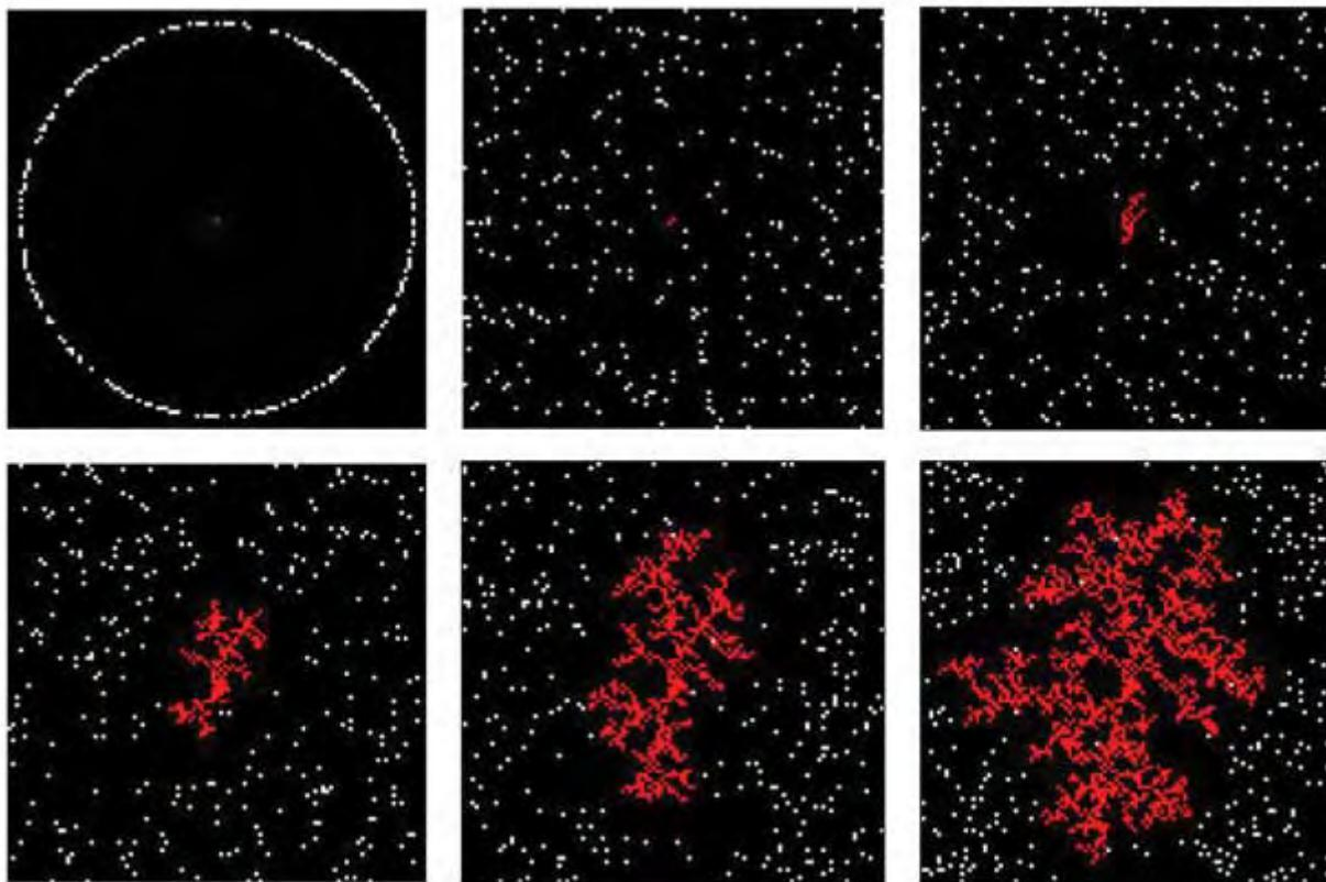
Figure 5: Generating Clustered City Growth Using Diffusion-Limited Aggregation
