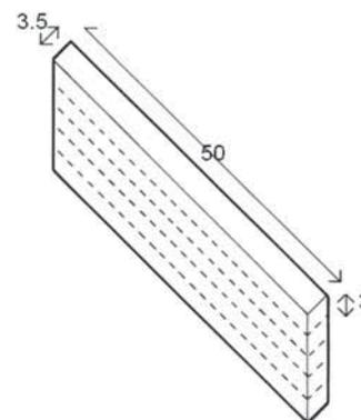
**Figure 9** Five-storey building block with depth 3.5 m, length 50 m and storey height 3 m. This has the same volume as the block shown in Figure 7
