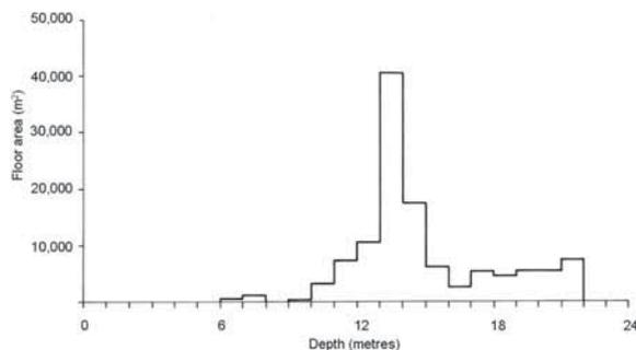
**Figure 10** Plan depths of 19 office buildings in Swindon, UK, from a survey reported in Steadman *et al.* (1993). The graph shows the total floor area ( $m^2$ ) in the sample with the given plan depth (m)
