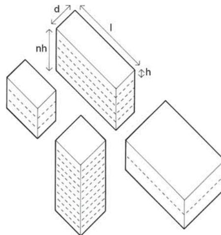
**Figure 4** Building block with depth  $d$ , length  $l$ , number of storeys  $n$  and storey height  $h$
