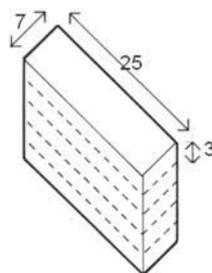
**Figure 7** Five-storey building block with depth 7 m, length 25 m and storey height 3 m. The value of  $V/W$  (discounting the end walls) is 3.5
