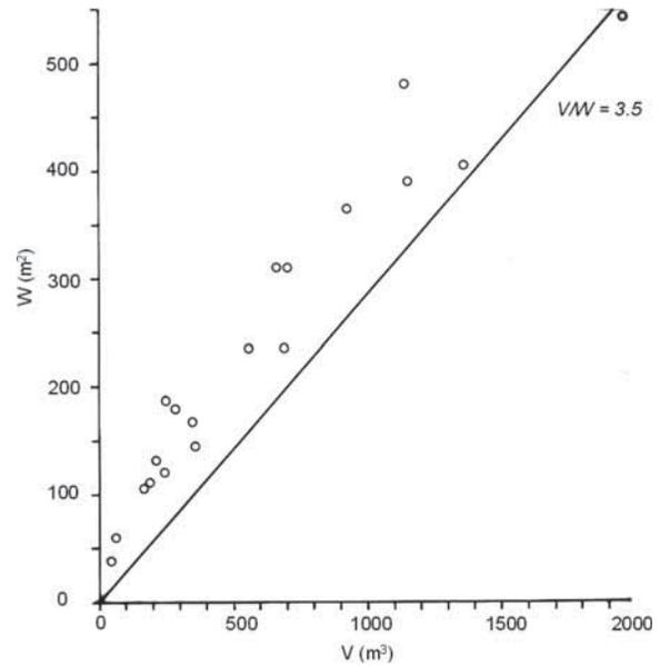
**Figure 5** Measurements of wall area  $W$  and volume  $V$  for the sample of small residential buildings given by Bon (1972a) (compare with Figure 2). This graph shows actual values for the smaller buildings. The heavy line marks a value of 3.5 for the ratio  $V/W$ , implying a plan depth of around 7 m. Some of these dwellings may be shallower than 7 m
