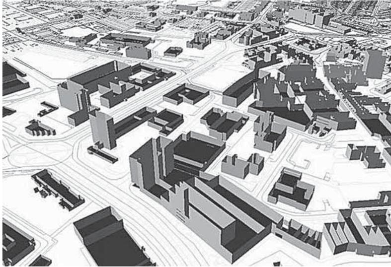
**Figure 11** Buildings in Swindon, UK, modelled in ArcView GIS, with internal plan contours offset from the window walls at 1 m spacing. The 1 m bands are coloured in darker shades with increasing distance from the windows
