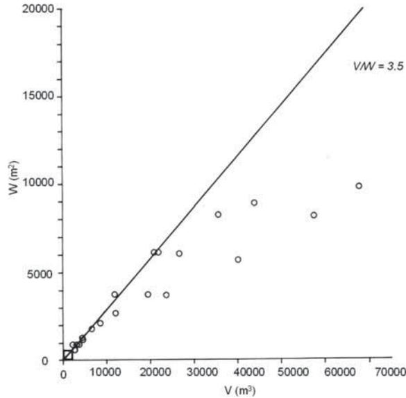
**Figure 6** Measurements of wall area  $W$  and volume  $V$  for the sample of large residential buildings given by Bon (1972a) (compare with Figure 2). This graph shows actual values for the larger buildings. The heavy line marks a value of 3.5 for the ratio, implying a plan depth of around 7 m. Many of these dwellings are deeper than 7 m
