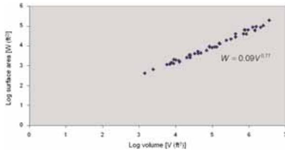
**Figure 2** Measurements of wall area  $W$  and volume  $V$  for a sample of 40 residential buildings, replotted on a log–log scale from data given by Bon (1972a)
