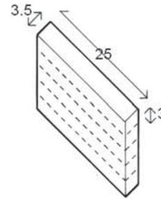
**Figure 8** Five-storey building block with depth 3.5 m, length 25 m and storey height 3 m. The value of  $V/W$  (discounting the end walls) is 1.75
