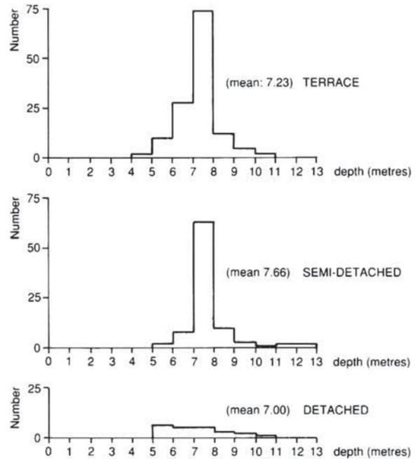
**Figure 3** Statistics from a representative survey of 300 dwellings in Cambridge, UK, made by Brown and Steadman (1991) showing distributions of overall plan depth (m) for terrace, semi-detached and detached houses
